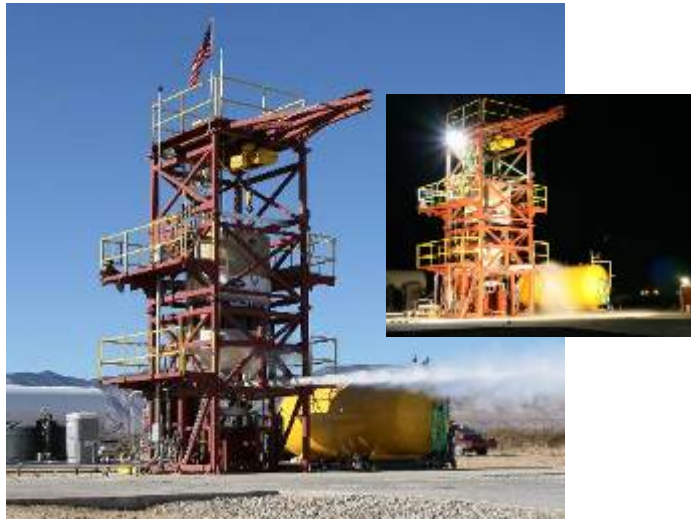
Liquid Oxygen (LOX) Cold Flow and Conditioning Tests on VTS
