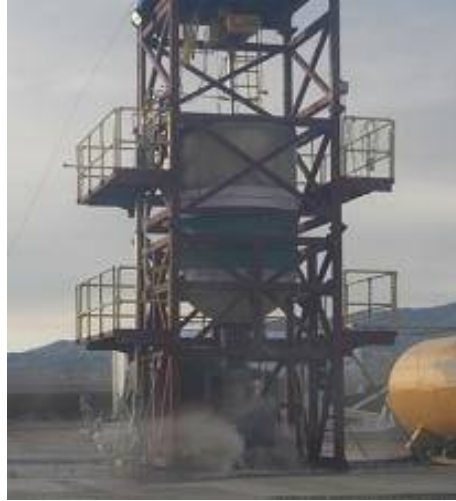
Facility Checkout Test Fire (10 seconds) on Vertical Test Stand (VTS)
