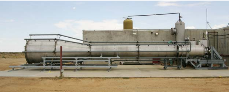
Test Stand Configured with Eductor for High Altitude Engine Tests
