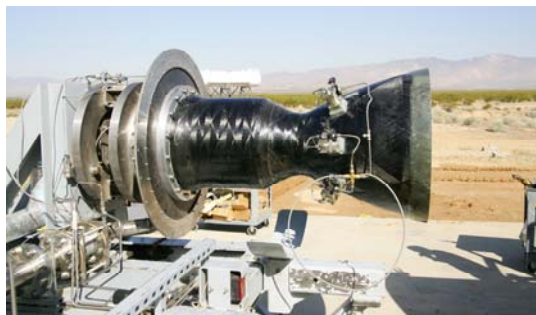
QuickReach™ Stage 2 Engine on Test Stand with 8:1 Nozzle
