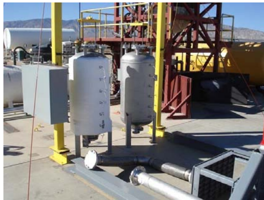
Plumbing in Place in the Propellant Lines on Horizontal Test Stand (HTS)
