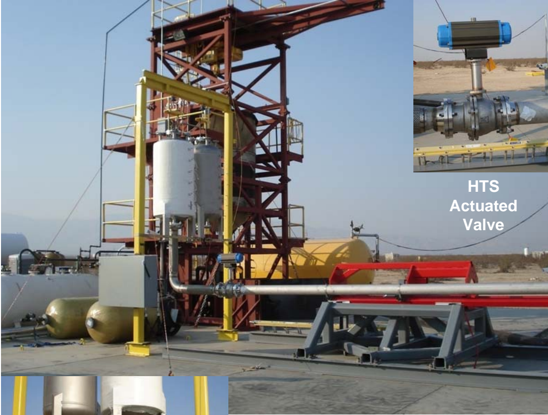
Plumbing in Place in the Propellant Lines on Horizontal Test Stand (HTS)
