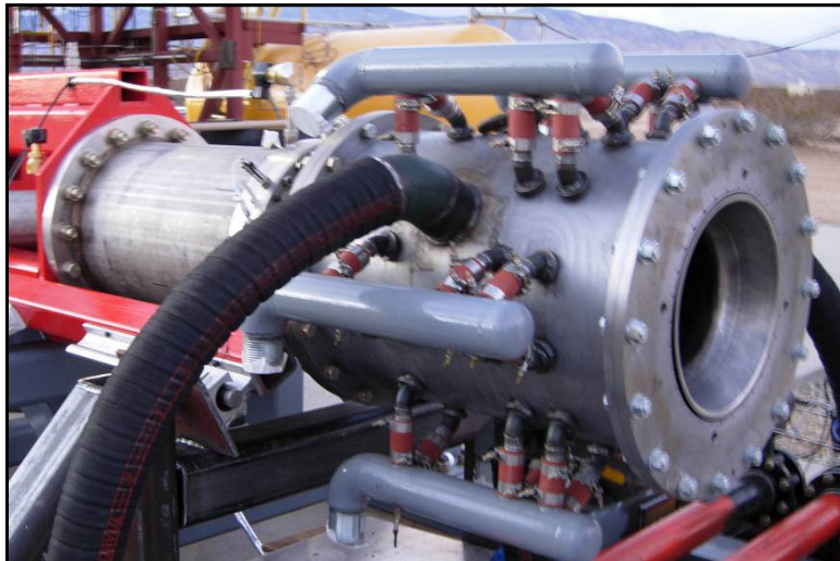
Use of the Water-Cooled Test Engine enables Rapid and Repeated Testing of the Engine at Minimum Cost.
