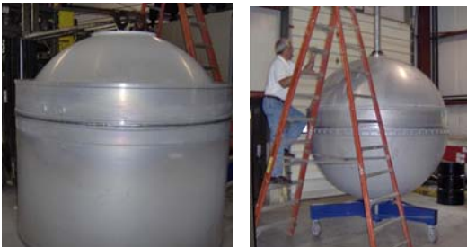
Propane tank & LOX tank completed
